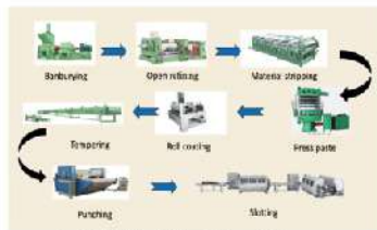
Figure 1 BBL WPC resilient flooring tile manufacturing process
